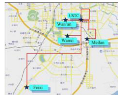
Metropolitan all-pass quantum communication network constitutes 4 nodes
